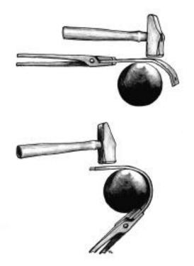
8. Manipulation of stock for bending on the horn.
