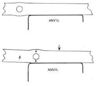
5. Proper placement of the bar.
