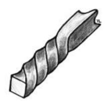
11. Forging dynamics of twisting.
