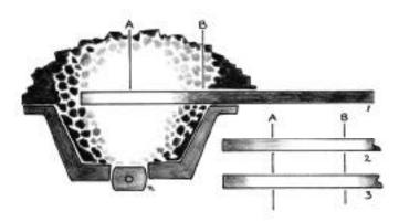
4. Measuring and heating the bar.
