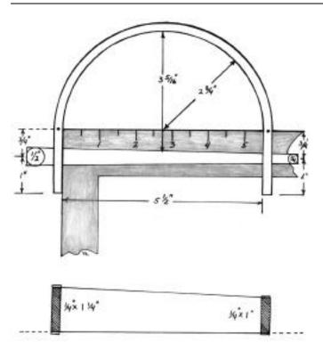
9. A square can be used to assure that the curve begins and ends properly, to locate a center to check the curve, and to check that the straight ends are parallel. The sides of the curved bar should lie evenly on a flat surface except for the swelling around the punched holes.
