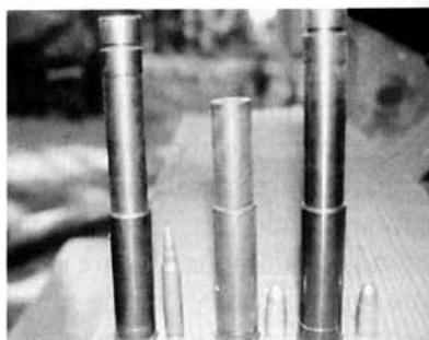
Twelve-gauge shotgun inserts, having their own stubby barrels, accurately fire 9mm pistol and .223 rounds.
