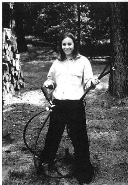
A small electric-drill pump is essential to pull fuel from large storage tanks.
