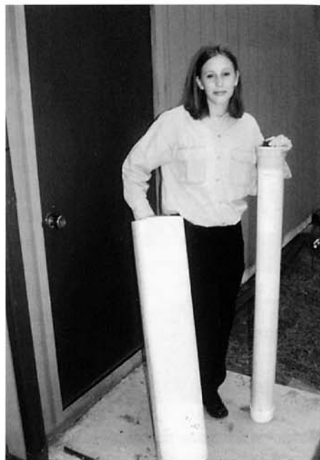
Sturdy cache tubes can be made using 4- and 8-inch SDR pipe.
