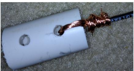
Either purchase two dogbone insulators, or cut two 2" sections from a piece of 1/2" or 3/4" PVC and drill two 1/4" holes near one end and two near the other end of each PVC section.
