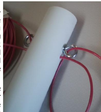
Tie-wrap each 66' wire onto itself around its eyebolt using two 15" zip-ties each, to provide a secure strain relief. Slip the other end of each of the 66' wires through two end holes of a dogbone insulator, such that the length from the eyebolt to the dogbone is 58' 6", then wrap the remaining wire onto itself, but do not cut any of the wire, to allow for tuning. Repeat with the 34' wires, to 30' 11". Repeat with the 19' wires, to 15' 8". Repeat with the 11' wires, to 7' 10".
